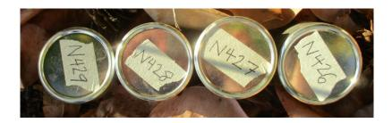
These tins were used for measuring soil moisture content and bulk density at Nymph Point Park. The leaves shown on the tins are reflections from the Arbutus tree above.
