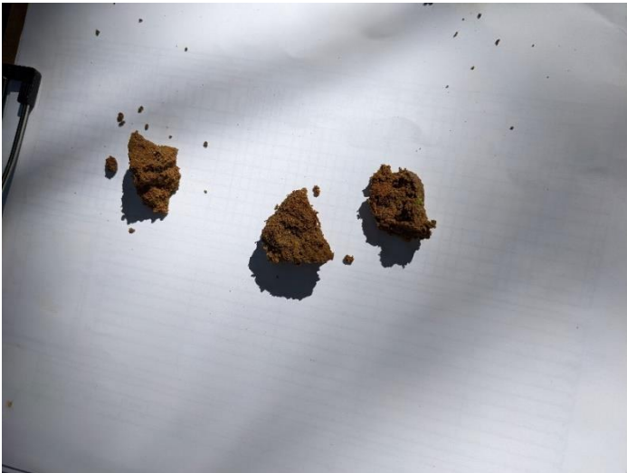
Figure 20 Slight cementation with iron deposits
