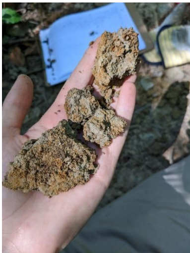
Figure 8 Prominent mottling in the C layer
